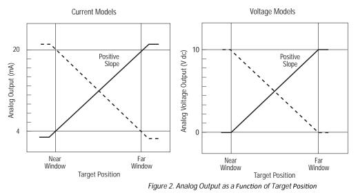
Note: The linear analog output tracks slightly past each window limit (from 3.8 mA to 20.5 mA).
