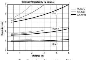
Figure 3. Resolution/Repeatability vs Distance
