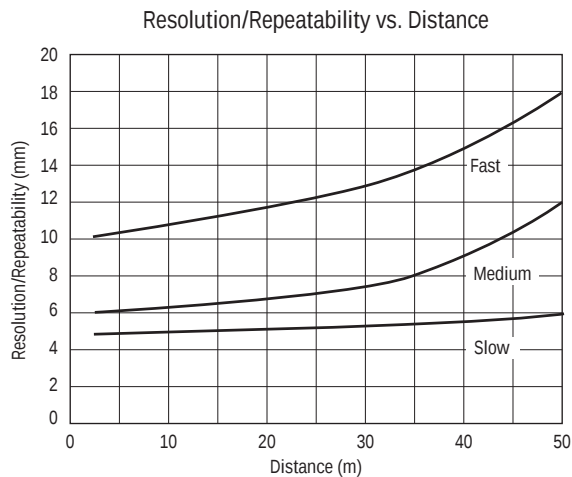
Figure 3. LT3 resolution/repeatability (retroreflective mode)
