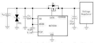
The next criterion is that the absolute maximum rating of Anode to Cathode reverse voltage of the MX74700(-100V) and the maximum V<sub>DS</sub> rating MOSFET are not exceeded. In the design example, 100V rated MOSFET is chosen and maximum limit on the cathode to anode voltage is 100V.
