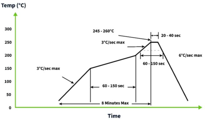
\*Temperatures listed within a tolerance of +/- 10º C
