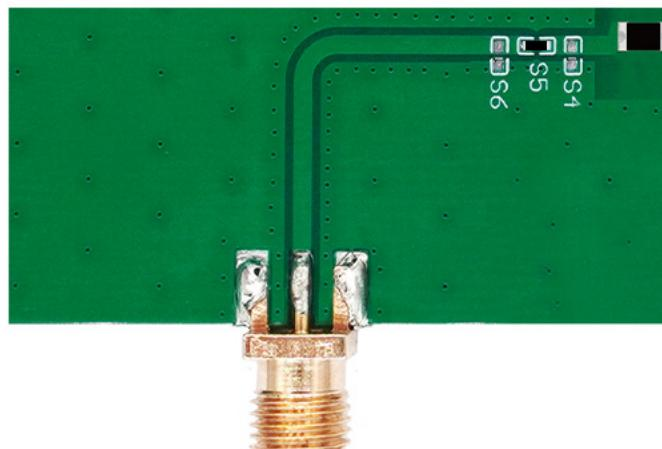
It's strongly recommended to place the antenna near the edge of the board. Maximum antenna performance is achieved by placing the antenna towards one of the corners of the PCB and with the feed point of the antenna as close to same corner of the PCB as possible.
