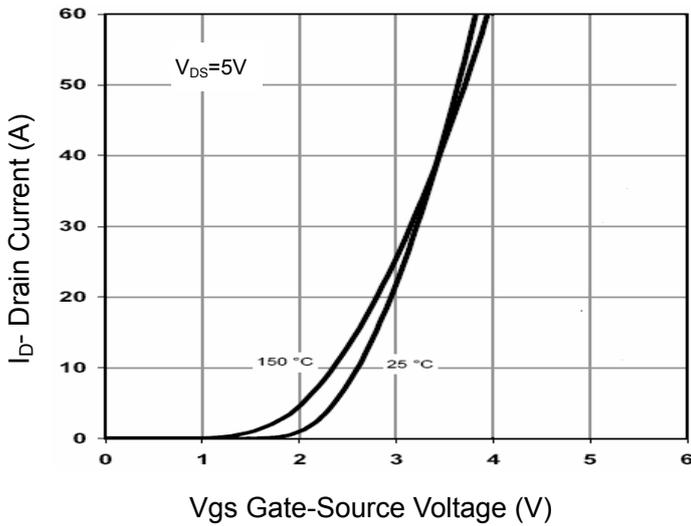
Figure 2 Transfer Characteristics
