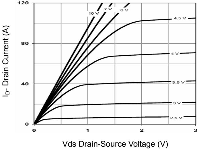
Figure 1 Output Characteristics
