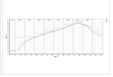
Remarks: All temperatures referred are measured on the surface of the package body.
