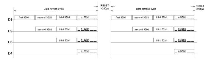
Note: The data of D1 is send by MCU, and D2, D3, D4 through IC internal reshaping amplification to transmit.
