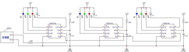
2. Supply voltage=12V (Each channel drives 3 LEDs)
