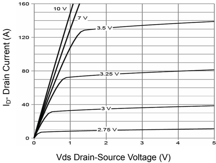
Figure 1 Output Characteristics
