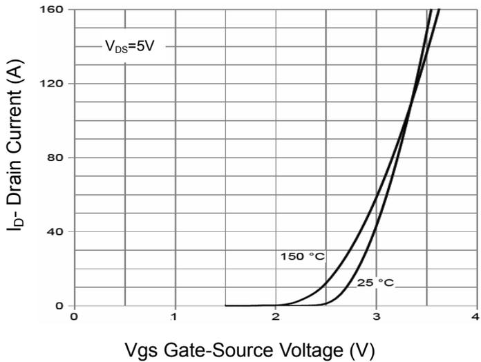
Figure 2 Transfer Characteristics
