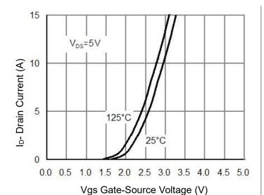
**Figure 7 Transfer Characteristics**
