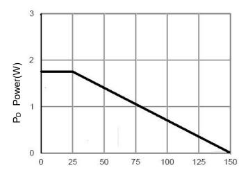
T<sub>J</sub>-Junction Temperature(°C) **Figure 3 Power Dissipation**
