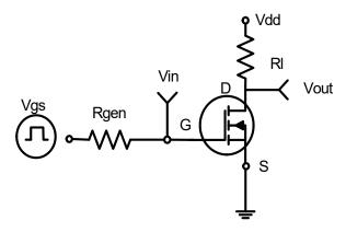
**Figure 1:Switching Test Circuit**
