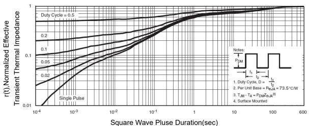
**Figure 14 Normalized Maximum Transient Thermal Impedance**
