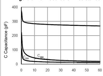
Figure 10 Capacitance vs Vds
