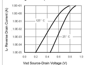
Figure 12 Source- Drain Diode Forward
