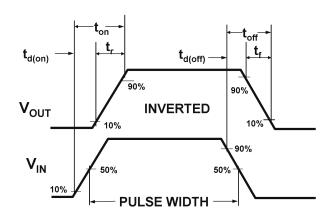
Figure 2:Switching Waveforms
