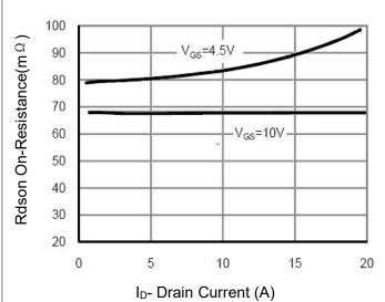
Figure 6 Drain-Source On-Resistance
