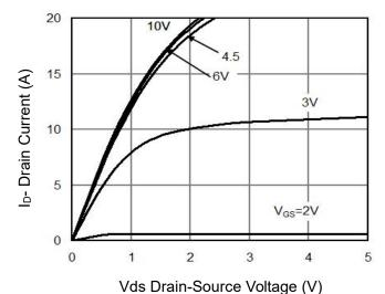
Figure 5 Output Characteristics
