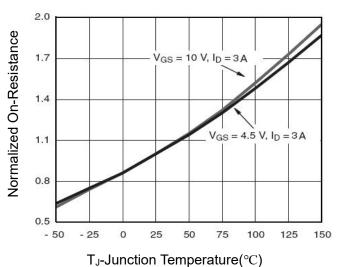
Figure 8 Drain-Source On-Resistance
