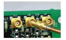
• Quick connect/disconnect snap-on mating reduces installation time.
