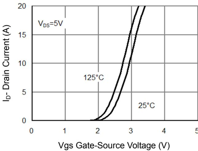
Figure 2 Transfer Characteristics
