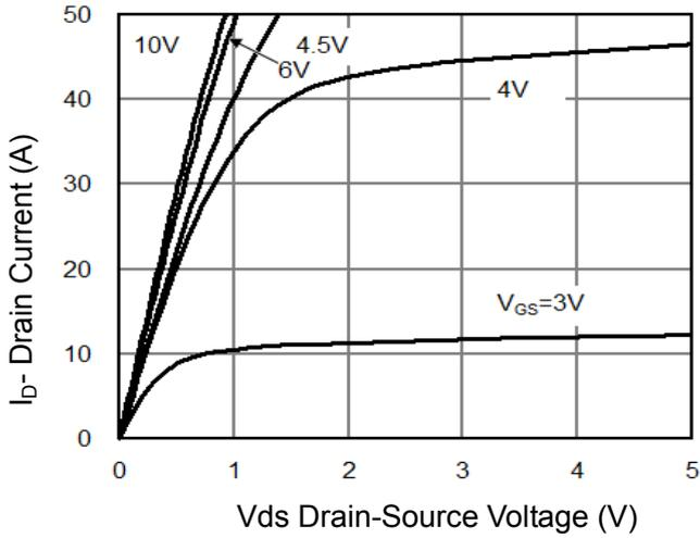
Figure 1 Output Characteristics
