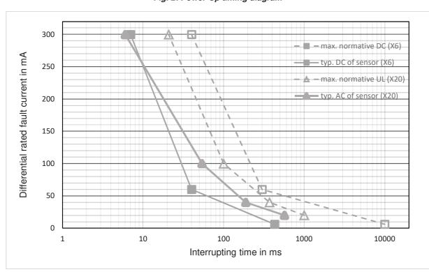
Fig. 3: Interrupting Time according to IEC62752 (E)-1:2016, UL2231-2 Ed.2 and typical values of sensor
