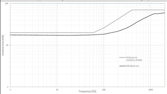
Fig. 4:UL2231 response value over frequency
