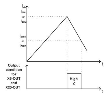
Fig. 1: Meaning of switching recovery level
