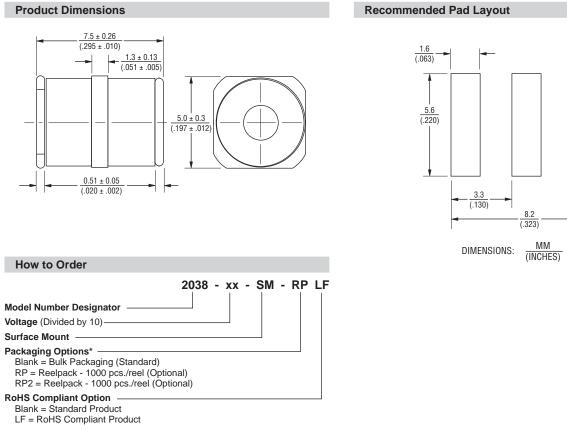
\*The optional -RP & -RP2 reelpacks contain 1000 pcs./reel. The reels are 330 mm (13 inches) in diameter. The -RP reelpack is 18 mm (0.71 inches) wide. The -RP2 reelpack is 26 mm (1.02 inches) wide.
