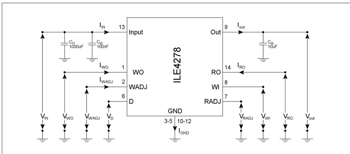
Figure 2. Test circuit
