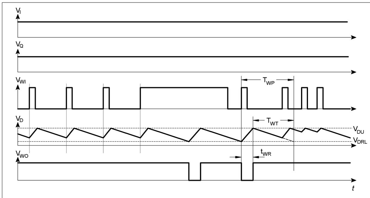
**Figure 5. Timing of the Watchdog Function**
