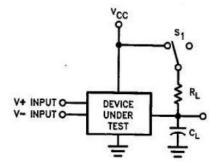
CL = Includes load and test jig capacitance.
