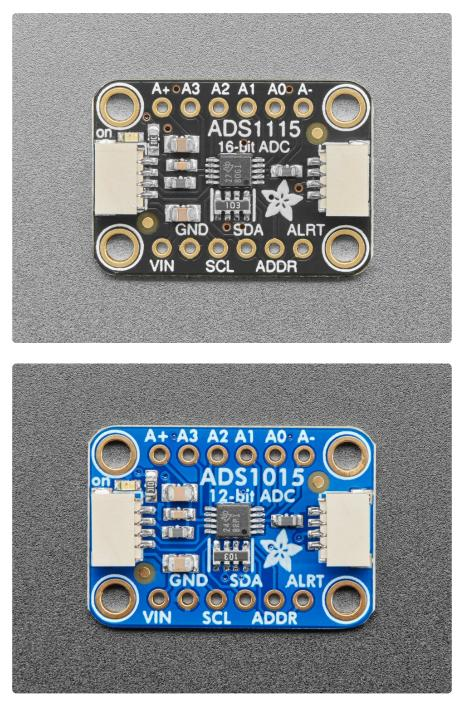
The ADS1115 and ADS1015 4-channel breakout boards are perfect for adding highresolution analog to digital conversion to any microprocessor-based project. These boards can run with power and logic signals between 2v to 5v, so they are compatible with all common 3.3v and 5v processors. As many of 4 of these boards can be controlled from the same 2-wire I2C bus, giving you up to 16 single-ended or 8 differential channels. A programmable gain amplifier provides up to x16 gain for small signals.
