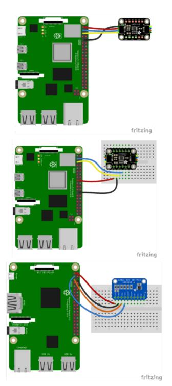
Pi 3V (red wire in STEMMA QT version) to ADS1x15 VDD - Remember the maximum input voltage to any ADC channel cannot exceed this VDD 3V value! Pi GND (black wire in STEMMA QT version) to ADS1x15 GND Pi SCL (yellow wire in STEMMA QT version) to ADS1x15 SCL Pi SDA (blue wire in STEMMA QT version) to ADS1x15 SDA
