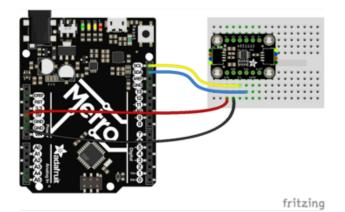
Connect SCL on the Metro to SCL (yellow wire in STEMMA QT version) on the ADS1x15 Connect SDA on the Metro to SDA (blue wire in STEMMA QT version) on the ADS1x15 Connect GND on the Metro to GND (black wire in STEMMA QT version) on the ADS1x15 Connect 5V on the Arduino/Metro to VIN (red wire in STEMMA QT version) on the ADS1x15
