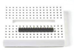
Prepare the header strip Cut the supplied header strip to length and insert it long-pins-down in your breadboard to hold it for soldering.
