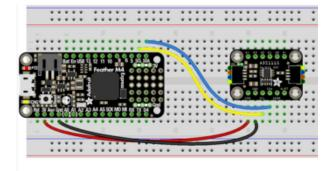
Board 3V (red wire in STEMMA QT version) to ADS1x15 VDD - Remember the maximum input voltage to any ADC channel cannot exceed this VDD 3V value! Board GND (black wire in STEMMA QT version) to ADS1x15 GND Board SCL (yellow wire in STEMMA QT version) to ADS1x15 SCL Board SDA (blue wire in STEMMA QT version) to ADS1x15 SDA
