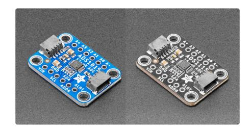
There are two versions of this board - the STEMMA QT version shown above, and the original header-only version shown below. Code works the same on both!
