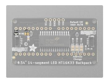
On LED - On the left side of the back of the board is a little green LED labeled On. This LED lights up when the board is successfully powered.
