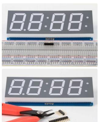
Cut the header strip to length if necessary and insert LONG pins down into the breadboard.
