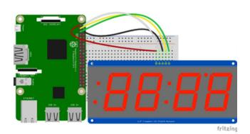
Raspberry Pi 3.3V to 7-Segment Display IO
