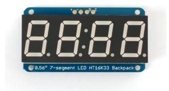
Remove the parts from packaging and place the LED matrix OVER the silkscreen side. DO NOT PUT THE DISPLAY ON UPSIDE DOWN OR IT WONT WORK!! Check the image below to make sure the 'decimal point' dots are on the bottom, matching the silkscreen.
