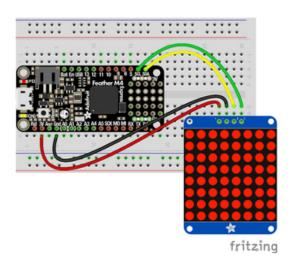
Microcontroller 3V to LED Matrix VIN
