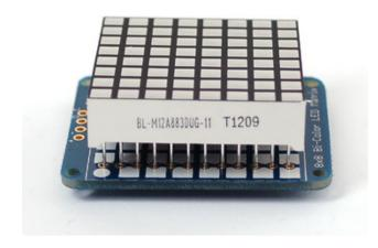
Remove the parts from packaging and place the LED matrix OVER the silkscreen side.
