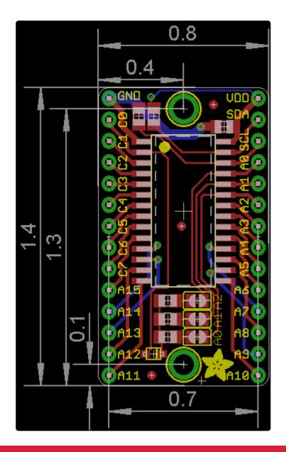
NOTE - The silkscreen labels for the AO/A2 header pins are swapped. The silkscreen labels for the solder pads are correct.
