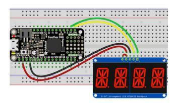
Microcontroller 3V to AlphaNumeric Display I2C VIN
