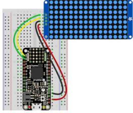
Microcontroller 3V to LED Matrix VIN
