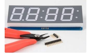
Cut the header strip to length if necessary and insert LONG pins down into the breadboard.
