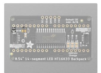
**On LED** - On the left side of the back of the board is a little green LED labeled **On**. This LED lights up when the board is successfully powered.
