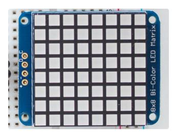
The default orientation for graphics commands on this display places pixel (0,0) at the top-left when the header is at the left and Adafruit logo at the right. To use the matrix as shown above (header at top, logo at bottom), call matrix.setRotation(3) before issuing graphics commands.
