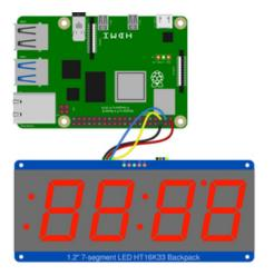
Raspberry Pi 3.3V to STEMMA QT red wire Raspberry Pi GND to STEMMA QT black wire
