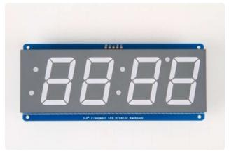
Remove the parts from packaging and place the LED matrix OVER the silkscreen side. DO NOT PUT THE DISPLAY ON UPSIDE DOWN OR IT WONT WORK!! Check the image below to make sure the 'decimal point' dots are in the same location as the ones on the silkscreen.
