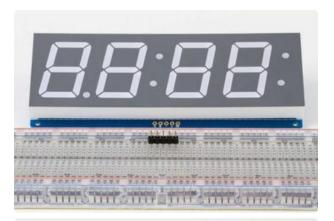
Cut the header strip to length if necessary and insert LONG pins down into the breadboard.
