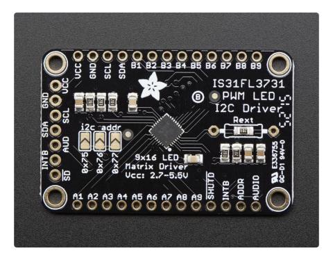
The IS31FL3731 will let you get back to that classic LED matrix look, with a nice upgrade! This I2C LED driver chip has the ability to PWM each individual LED in a 16x9 grid so you can have beautiful LED lighting effects, without a lot of pin twiddling. Simply tell the chip which LED on the grid you want lit, and what brightness and it's all taken care of for you.
