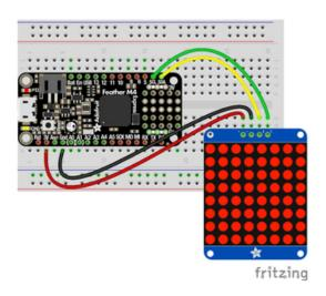
Microcontroller 3V to LED Matrix VIN
