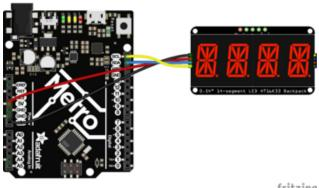
Board 5V to backpack Vio (red wire) Board GND to backpack GND (black wire) Board SCL to backpack SCL (yellow wire) Board SDA to backpack SDA (blue wire)
