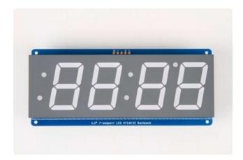
Remove the parts from packaging and place the LED matrix OVER the silkscreen side. DO NOT PUT THE DISPLAY ON UPSIDE DOWN OR IT WONT WORK!!
