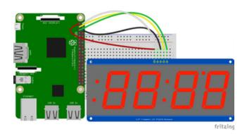
Raspberry Pi 3.3V to 7-Segment Display IO
