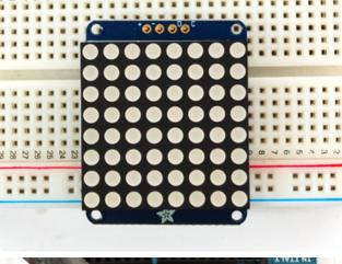
Place the soldered backpack on top of the header.
