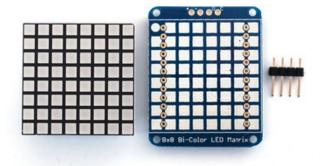
When you buy a pack from Adafruit, it comes with the fully tested and assembled backpack as well as a 8x8 matrix. You'll need to solder the matrix onto the backpack but its an easy task.
