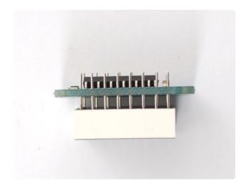
Remove the parts from packaging and place the LED matrix OVER the silkscreen side. It can go 'either way' - the matrix is symmetric so as long as it goes onto the front it will work in any orientation. Do not solder the matrix over the chip on the back of the backpack - it will not work then!
