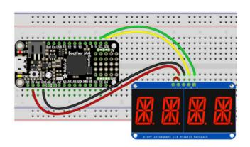
Microcontroller 3V to AlphaNumeric Display I2C VIN
