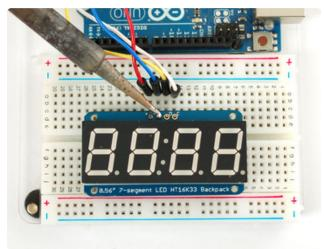
Place the soldered backpack on top of the header and Solder 'em!
