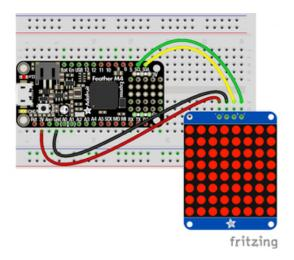
Microcontroller 3V to LED Matrix VIN
