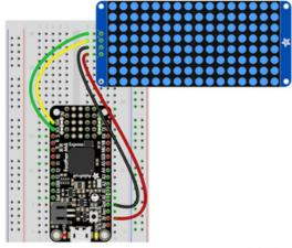
Microcontroller 3V to LED Matrix VIN
