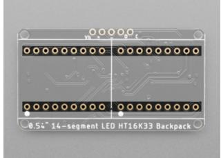
These two rows of through-hole pads are for soldering the alphanumeric LED displays onto the backpack. See the Assembly page (https://adafru.it/11dU) for details on attaching the displays properly.
