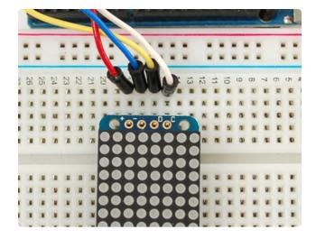
Place the soldered backpack on top of the header.
