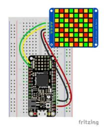
Microcontroller 3V to LED Matrix VIN
