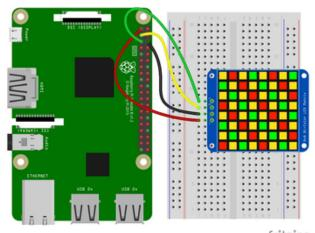
Raspberry Pi GND to LED Matrix GND Raspberry Pi SCL to LED Matrix SCL Raspberry Pi SDA to LED Matrix SDA
