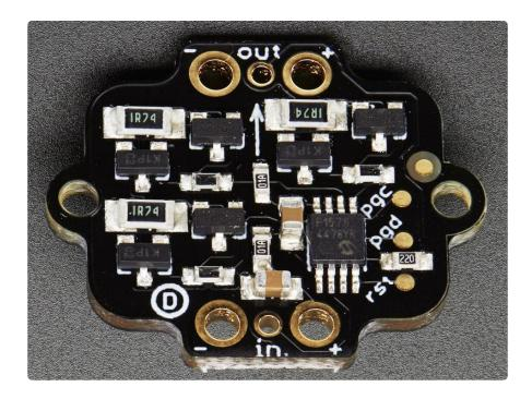
Pixie has two 'ports' - one for input and one for output. Both input and output ports have power pins:
