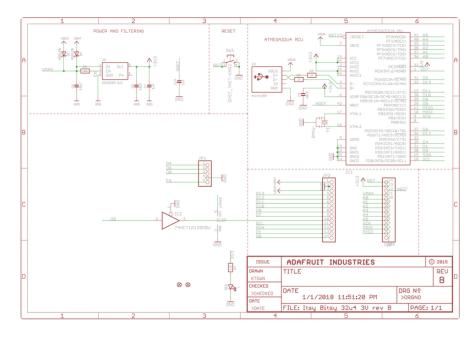
The 3.3V schematic regulator should be AP2112K-3.3
