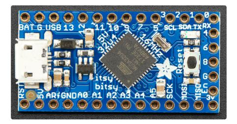
The pinouts for these are very similar except for the power pins which have different voltages!
