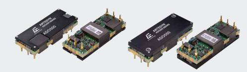
ADO500/550 series eighth-brick isolated DC-DC converters produce a single fully regulated 10 V output. Rated at 500/550 watts, these converters can deliver up to 55 amps output current and have no minimum load requirement. They have an input voltage range of 45 to 56 V and are primarily designed for use with standard 48 V supplies in computing and server applications, as well as regulated 48V supplies in communications equipment.
