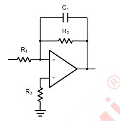
Figure 5. Low Pass Active Filte
