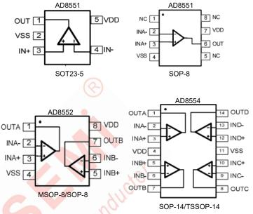
Figure 1. Pin Assignment Diagram
