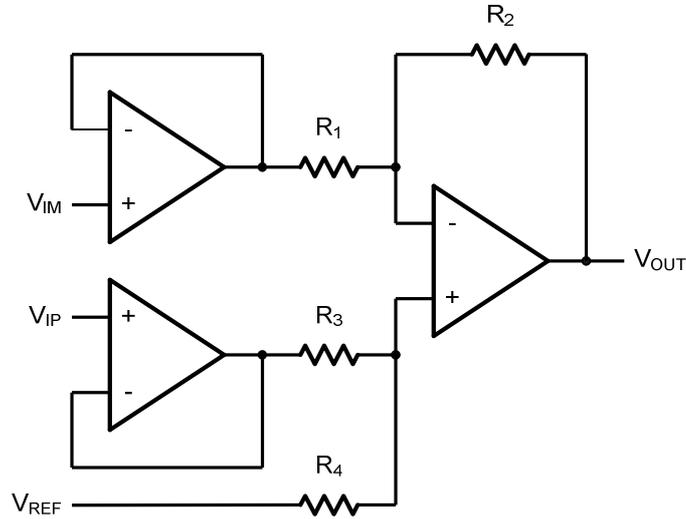
Figure 6. Instrument Amplifier
