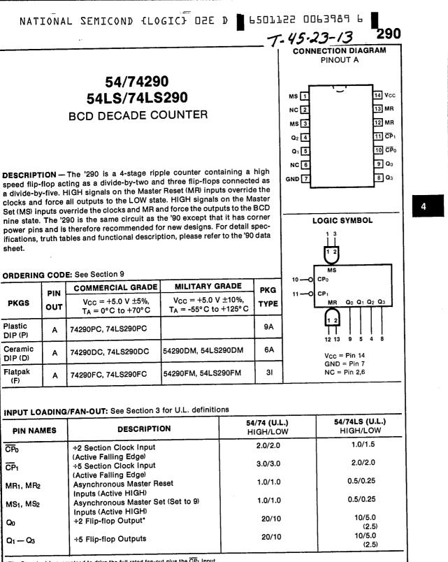
The Q<sub>0</sub> output is guaranteed to drive the full rated fan-out plus the  $\overline{CP}_1$  input.
