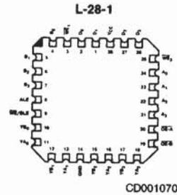
Note: Pin 1 is marked for orientation
