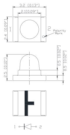
Units: mm / tolerance = +/-0.15mm
