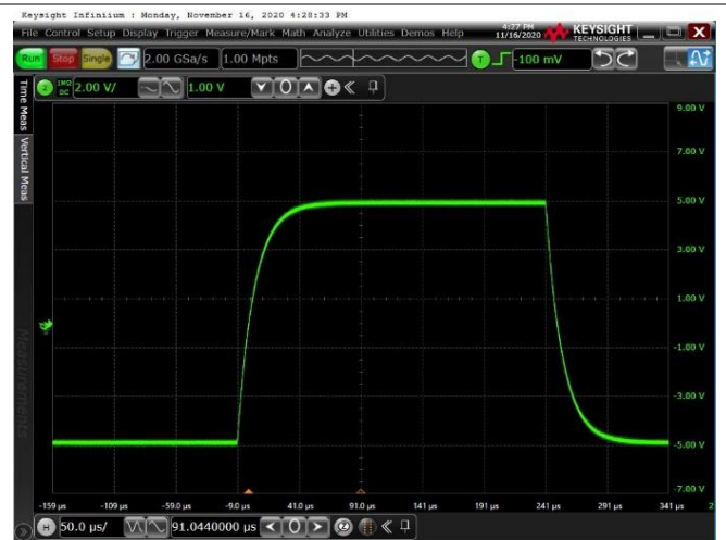
Voltage: 2V/div for Output, Time: 50us/div G=1000, VREF = GND; VIN=10mVPP, Load R=10K C=100pF
