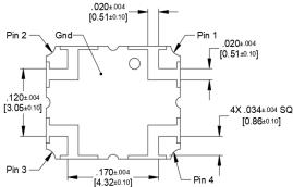
Dimensions are in Inches [Millimeters] Tolerances are Non-cumulative
