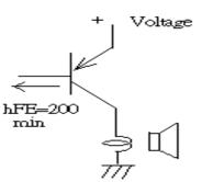
The base current Ib should high enough so that it saturates the collector current of the transistor with the CB load.
