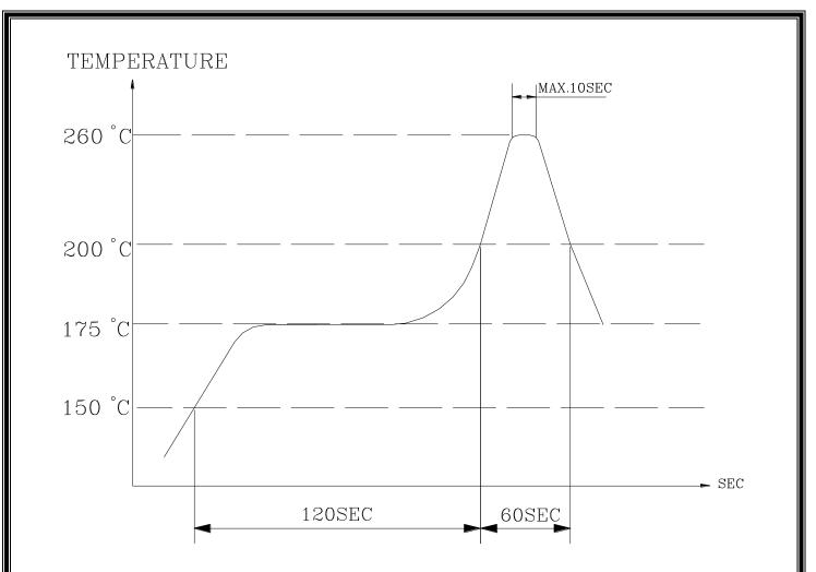
Heat resistant line (Used when heat resistant reliablity test is performed)
